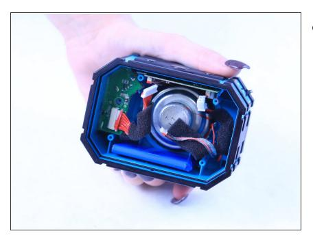
Unplug all wires that are connected to the motherboard.
