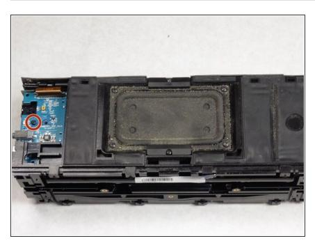
Remove the indicated T6 7.4 mm screw holding the auxiliary board in place.
