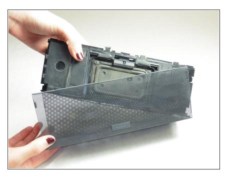
Once all eight screws are removed, pry the sides of the Jambox to lift the body from it's shell.
