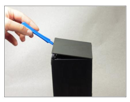
Remove both end caps by putting a plastic opening tool in the center of the seam. Work around the edges to pry the end caps off completely.
