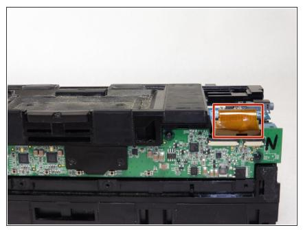
Remove the colored ribbon that connects the green button circuit board to the blue auxiliary board by using your finger to lift the small black tabs that clamp down the ribbon.
