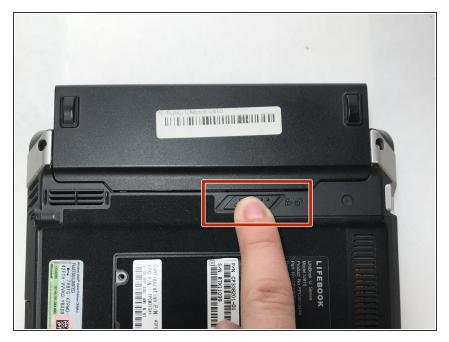
Push the latch to the right to release the battery.
