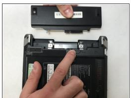
Hold the latch in the unlocked position and with your other hand pull the battery straight out from the back of the device.
