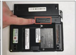
Flip the Lifebook so it's underside is showing and you see a small latch with the lock symbol on the right side.
