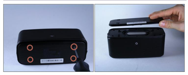
• Use a JIS #00 screwdriver to remove the four 3/32" screws that attach the base-plate to the speaker enclosure.
