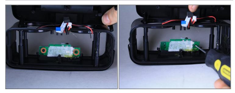
• Locate and remove the two 3/32" screws, indicated by red markers, that fix the motherboard to the speaker enclosure.
