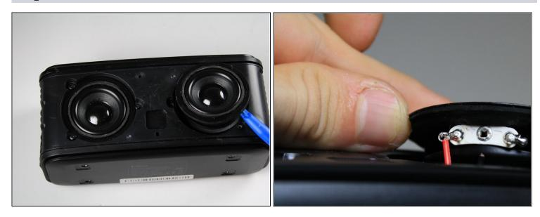
• Use the Plastic Opening Tool to gently lift the speaker enough to see the connected wires.
