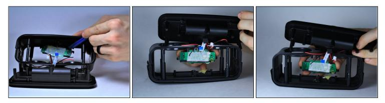
• Using the plastic opening tool, gently begin to pry the circuit card away from the speaker enclosure.
