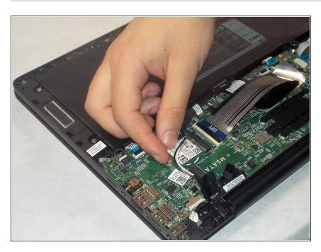
Disconnect the network card from motherboard socket.
