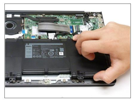
To remove the battery, lift up on one side to get your fingers underneath and lift away.
