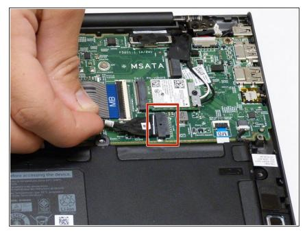
Use your fingers to remove the connecting cable to the battery unit.
