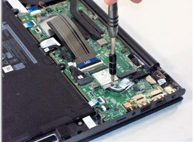
Use #1 Phillips screwdriver to remove the 1mm screw in the network card.
