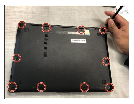
Remove the ten 10mm Phillips #0 screws on the back of the laptop.
