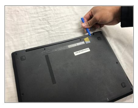
Use the iFixit opening tool along the edge of the laptop to pry open the back.
