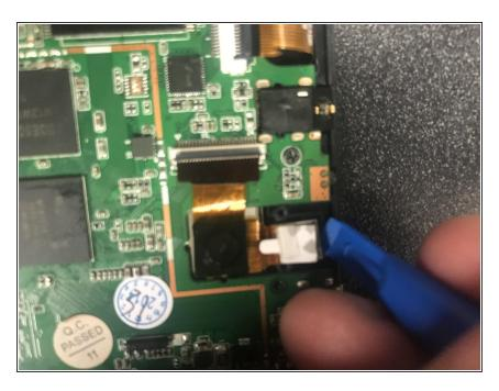
Now, carefully remove the front camera with the same wedge from step one, six, and eight.
