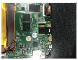
Use the J0 Phillps screw driver to unscrew the the two small screws on either side of the black peice.
