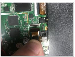
When the camera becomes loose, gental pull up and out to the right to silde the gold band out of the white and grey box.
