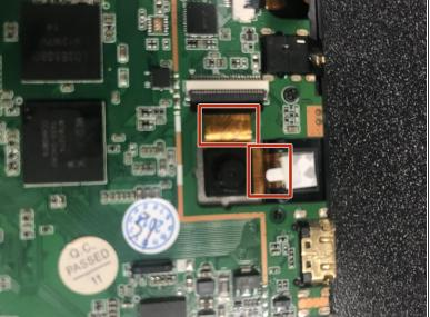
Pull the black camera cover off and locate the camera with two gold bands running off upwards and to the right.
