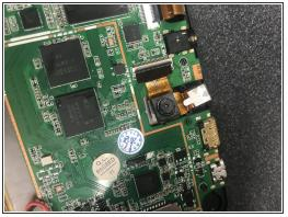
Use the same wedge used in step one and step six to go under the camera and carefully pry away from the sivler plating.
