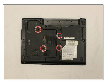
Unscrew the four 10 mm Phillips head screws circled in red in the picture using the Phillips 00 screwdriver.
