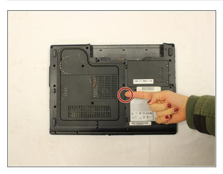
Put your pointer finger underneath the tab and lift up to remove the plastic cover.
