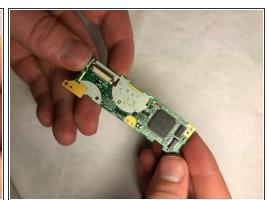
Pull the ribbon connected to the dial off the motherboard.
