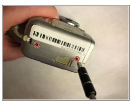
• Unscrew the eight 4mm long JIS #00 screws from the bottom, right side, and the left side.
