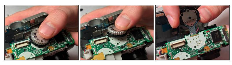
Push or slide the the top dial toward the backside of the camera to unclip from the motherboard.
