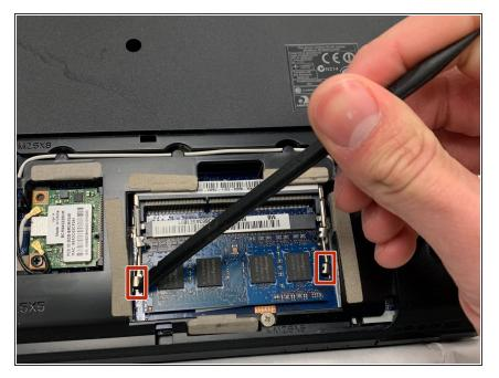
Push each of the two silver clips outward to release RAM board.
