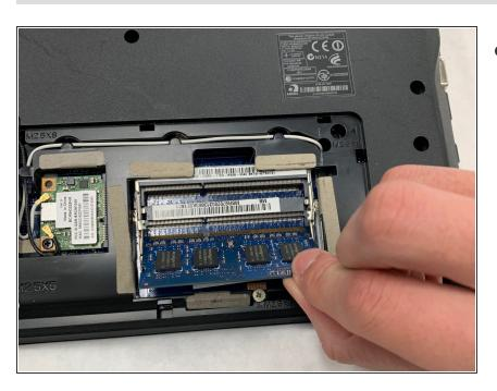
Lift RAM board out of its compartment.
