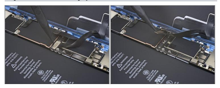
• Use the tip of a spudger to disconnect the display cable connector.
