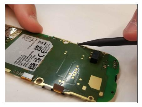
• Using your thumb, push the tab on the right side of the motherboard over to the right and then push downward to unclip the keyboard. It should fall away.
