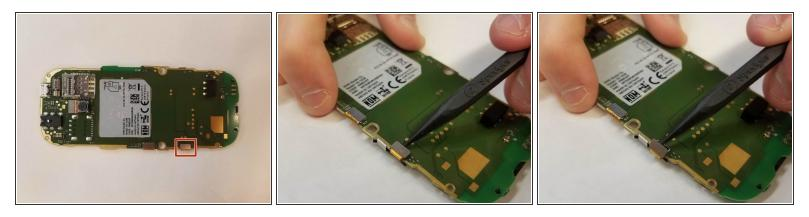
Using a spudger, unclip the bottom left snap to unplug the keyboard. The image shows the motherboard rotated 90 degrees counterclockwise
