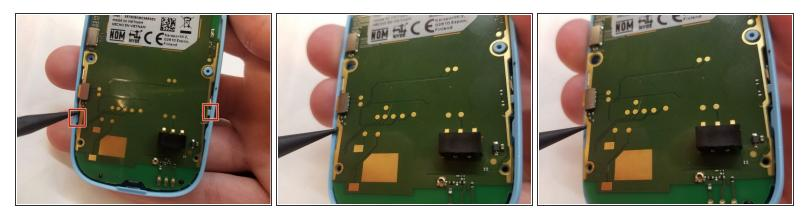
Use a spudger to simultaneously leverage the shell away and the motherboard up from the body of the shell.
