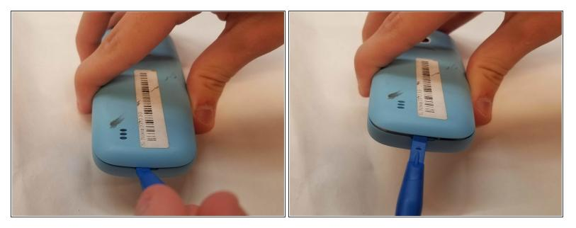
• Using the thumbtab molded on the bottom of the phone, pry the back cover off using either a fingernail or a plastic opening tool.
