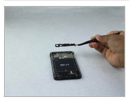
Using tweezers, remove the top black encasing of the camera.
