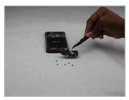
Remove the leftover screws using the PH000 screwdriver and release the bottom speaker holder piece.
