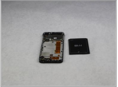
After fully removing the black speaker piece, the battery should be able to easily lift out with the aid
