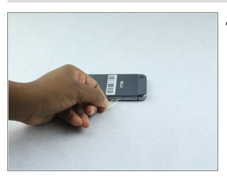
With the use of the SIM Card Eject Tool gently insert the tool into the hole.
