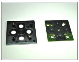
Using a the Metal Spudger, pry up the circuit board to reveal a rubber button panel.
