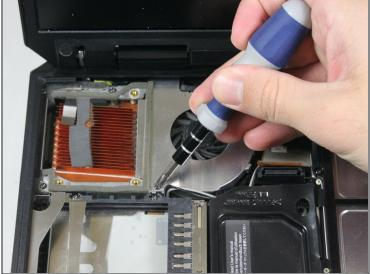
Remove the three 4 mm Phillips #0 screws securing the fan assembly.
