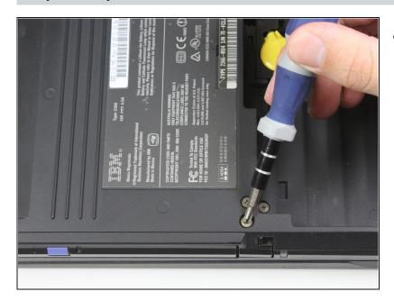
Locate the 4.8mm Phillips #0 screw on the far left of the ThinkPad, closest to the edge and above the battery, and unscrew it with a Phillips #0 screwdriver.
