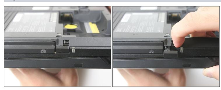
• On the side of the ThinkPad, locate a lock next to the optical drive. Use your fingernail to slide the lock to the right.
