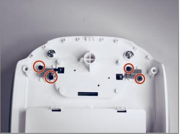
• Using a Phillips #00 screwdriver, remove the four screws on the inside of the panel. That will allow you to remove the buttons by gently lifting them with your hands.
