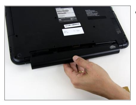
Pull the battery from the back of the laptop for removal from the laptop.
