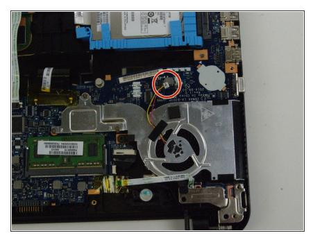
Disconnect the fan wire from the motherboard.
