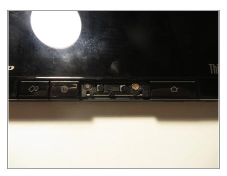
Remove the two 10mm Phillips #00 screws.
