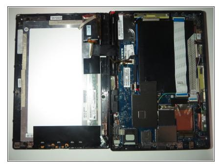
• Open the tablet screen to the left, making sure not to disconnect any of the wires connecting the screen to the tablet.
