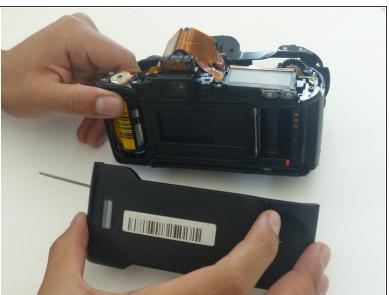
With a pair of tweezers or just your fingers, pull the rod completely out of the camera. The back latch should then completely detach from the camera.
