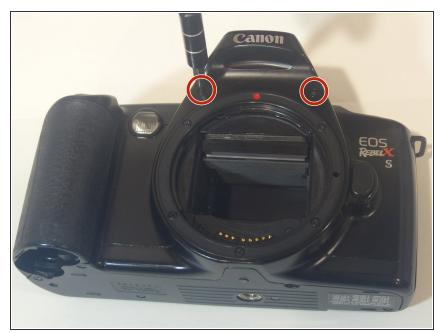
Using a Phillips #000 screwdriver, remove the two black screws shown in the picture that are both 6 mm in length and 1.25 mm in diameter.
