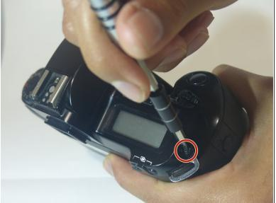
Using a PH000 screwdriver bit, remove the three black screws shown in the two pictures that are all 4 mm in length and 1 mm in diameter.
