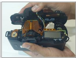
Using an opening tool (you can also use your nails, but try not to use something potentially damaging to the camera such as metal), separate the top cover from the rest of the camera!
