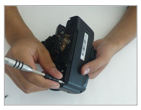
Once the front, top, and bottom covers have all been removed, it's time to remove the back latch! Using a paperclip or something similar (anything that's very skinny), push on the end of the skinny, silver, metal rod that vertically travels through the camera. Do this until enough of the rod pops out on the other side for the next step.
