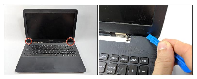
Remove the two plastic screw coverings from the bottom of the screen panel.
