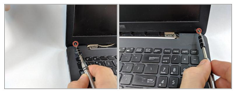
Remove the two 4.6mm screws using the Phillips #0 screwdriver.
