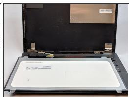
Carefully, lay screen down on the keyboard.
