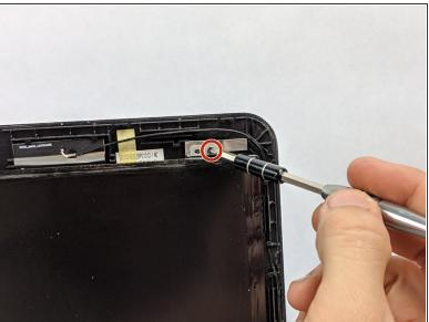
Remove the two 4.6mm screws holding screen in place.
