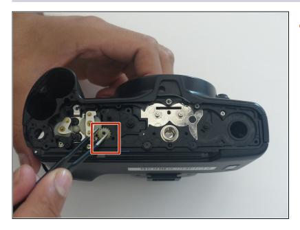
• Remove the gear with tweezers or fingers.
