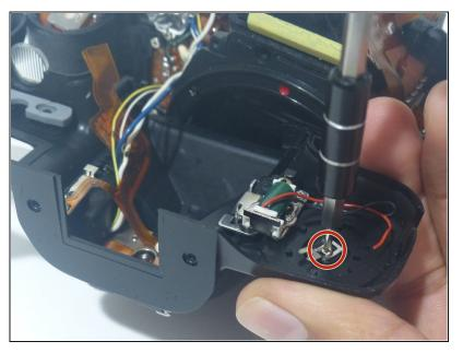
Using a PH000 screwdriver bit, remove the silver screw circled in the picture, which is 3 mm in length and 1 mm in diameter.
