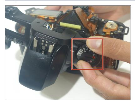
Locate the camera dial (surrounded by a red square) and turn the top cover of the camera upside down for access to the screw underneath the dial.
