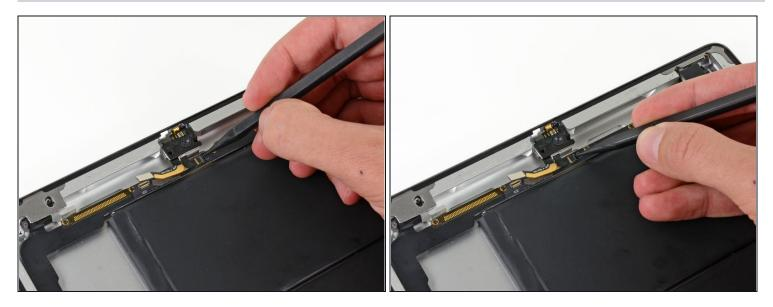
• Using the tip of a spudger, flip up the retaining flap on the microphone cable ZIF connector.
