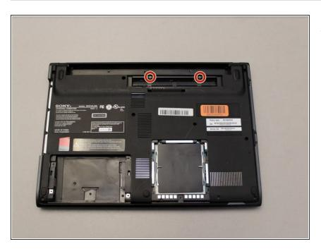
Remove the two 5 mm Phillips #0 screws from the bottom of the laptop.
