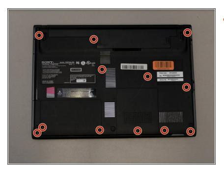
Remove the twelve 5 mm Phillips #0 screws from the bottom of the laptop.
