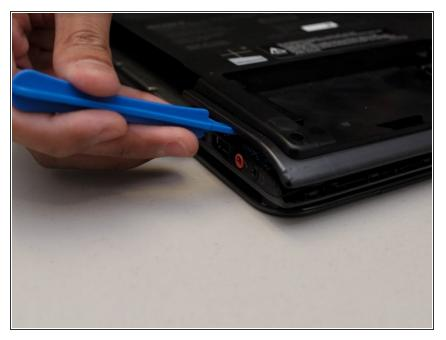
Using the plastic prying tools, go around the edge of the bottom of the laptop to release the cover.
