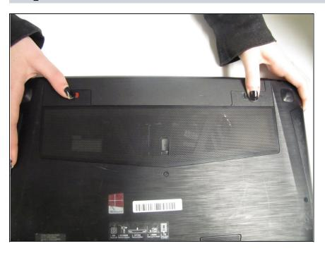
Move the latches to the unlocked position.
