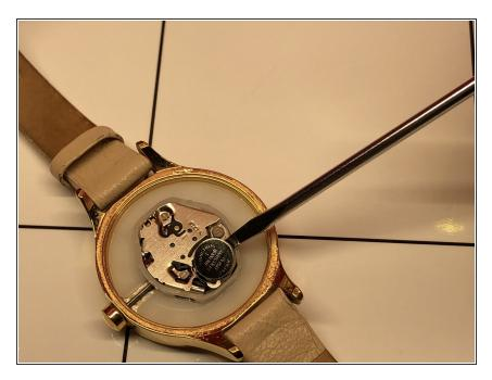
• While securing the inside of the watch with a finger or thumb, gently pry out the battery.
