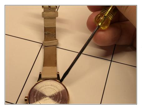
Pick a location that is by the band so that if you make any scratches they will be less obvious when you are done. Place the screwdriver between the frame and the back cover. Gently tap the back of the screwdriver with a small hammer or whatever you have around. Do not use your hand!
