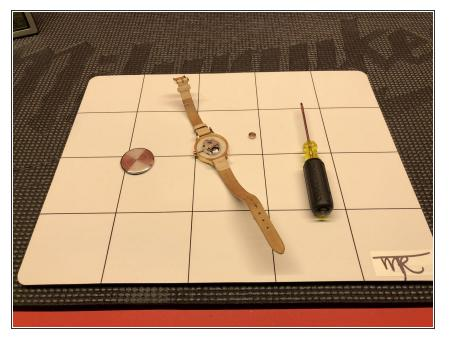
Insert a new battery. Line up the cover in the correct position. Keep the notch lined up with the winding screw. Secure the back to the frame by applying equal pressure and squeezing the two parts together.
