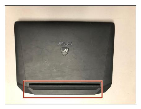
Gently pry the back hinge cover piece away from the device.
