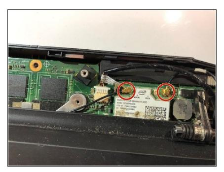
Remove tape and gently pull up on golden cap connectors to disconnect them.
