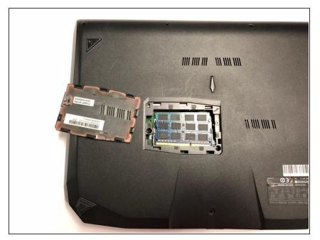
Remove the RAM cover by lifting the screw cover and pulling away firmly.
