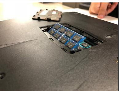
Push outwards on the clips to release the RAM stick. The stick should pop up at an angle.
