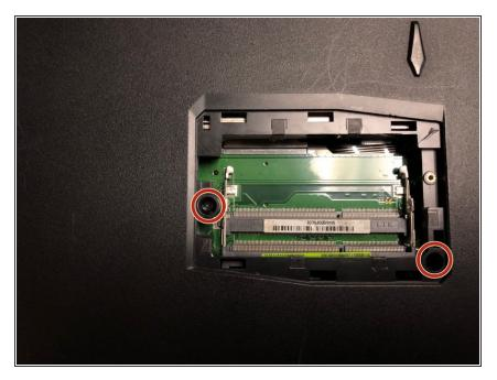
Remove the two screws from underneath the RAM cover.
