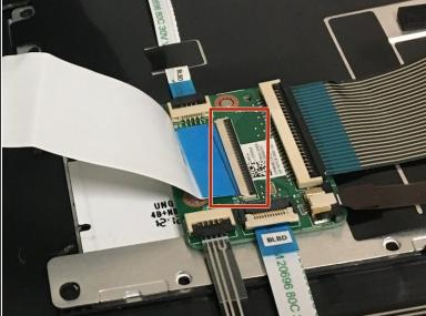
Detach the ribbon cable by releasing the clip
