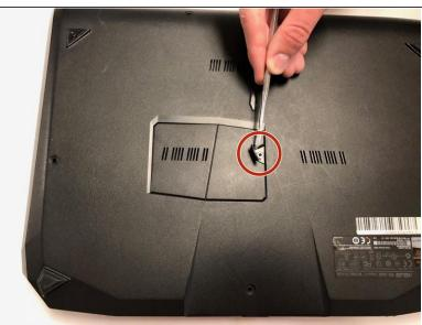
Lift the screw cover and remove the screw using a Phillips #0 screwdriver.
