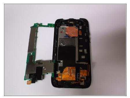
• Remove the motherboard without breaking it by placing it to the side. It will still be attached to the phone.
