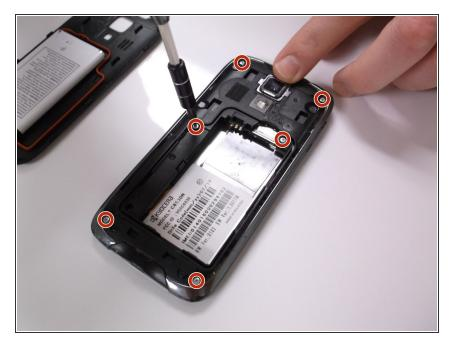
Use a PH0 screwdriver to remove the 6 screws which are holding the panel in the phone.
