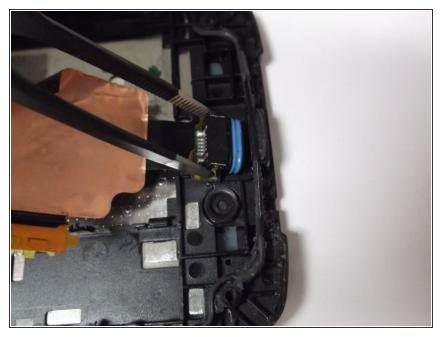
• Using force, remove the charging port from the charging slot.
