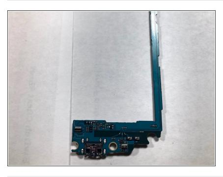
Once the logic board is stripped of the cameras, replace the logic board.
