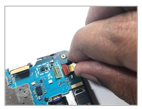
Once the camera is out of the housing, disconnect the camera from the logic board.
