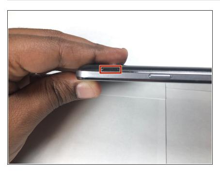
Locate the side notch that allows you to open the back casing.
