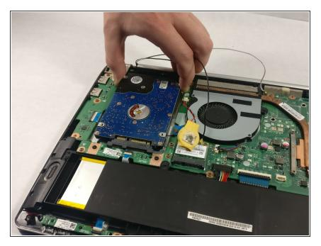
• Slide the hard drive out of the SATA port and remove it from the device.
