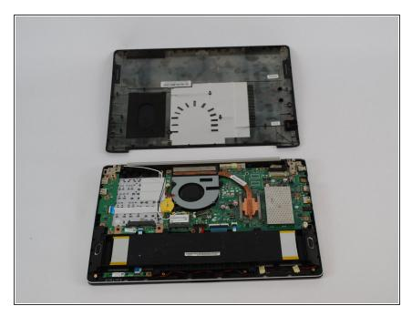
• Lift off the cover and remove the back cover from the device.
