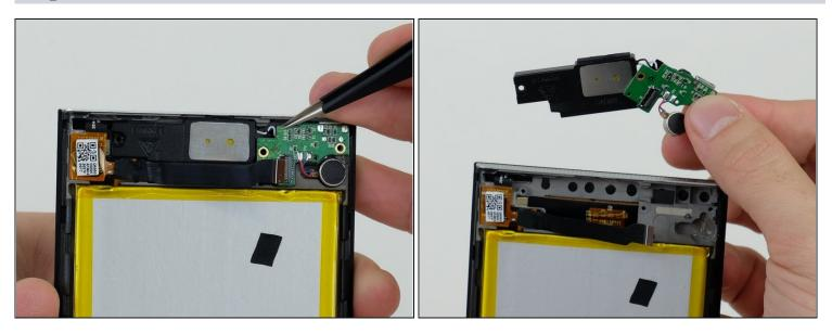
• Using the tweezers, grab a hold of the Micro USB assembly and gently remove it from the device.
