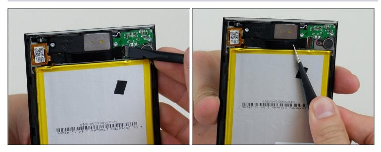
$\triangle$  The black ribbon can be easily damaged during this step, so proceed with caution.
