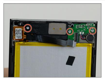
Remove all three 3mm-long silver screws using the T5 Torx screwdriver.
