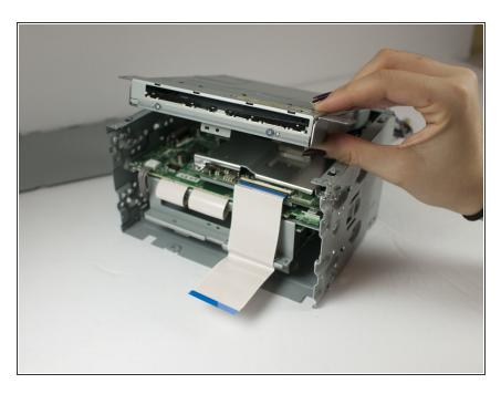
After removing all screws and top panel, lift up disc drive from steel enclosure.
