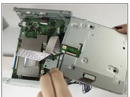
Gently pull to remove the electrical connector from disc drive.
