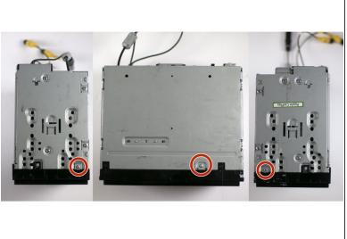
• Remove three steel-finish, pan-head, 1/64 x 3/16" machine screws identified in the photograph, using the Phillips #0 screwdriver.
