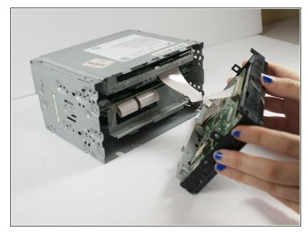
Gently remove the front panel from the steel enclosure.
