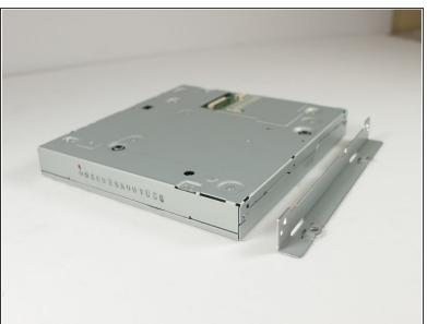
Remove 2 pan-head, 1/64 x 3/16" machine screws using a Phillips #0 screwdriver.
