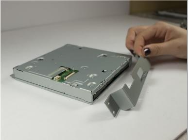
• Remove 2 pan-head, 1/64 x 3/16" machine screws using a Phillips #0 screwdriver.
