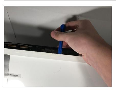
Use the plastic opening tool to pry open the white part away from the screen.
