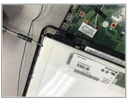
Remove the eight total screws (4 on each side) that are on the side of the white part on the back of the screen.
