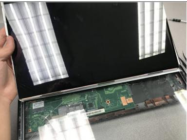
Pull the white part out and pull out the rest of the screen.
