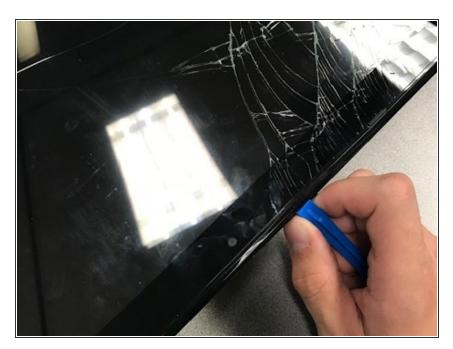
Insert the plastic opening tool on the side of the screen and slide it all the way around to open the screen up.
