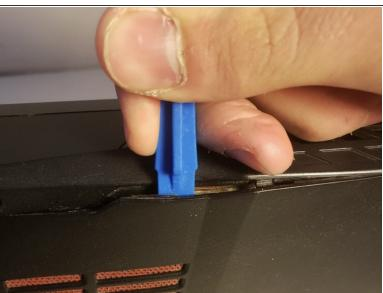
Insert the plastic opening tool into the back plate of the laptop and lightly pry it up.
