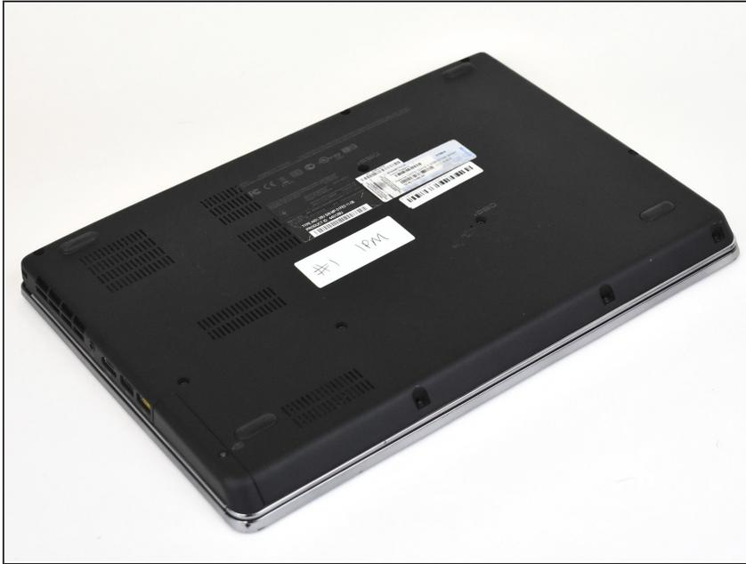
**⚠** There is no external access to the battery. Please make sure the at the battery has been drained or disabled through BIOS before beginning.
