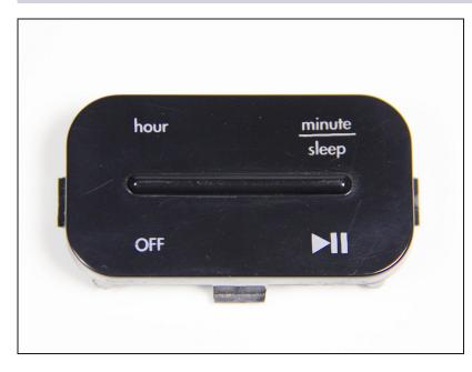
Replace your cracked or otherwise broken button with the new button.
