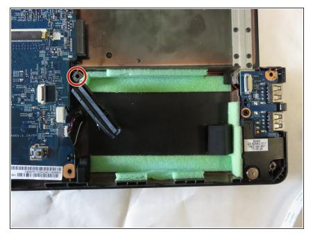
Remove the hard drive screw using Phillips #0 Screwdriver.
