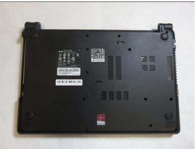
Remove nineteen screws from the back panel using a Phillips #0 Screwdriver.
