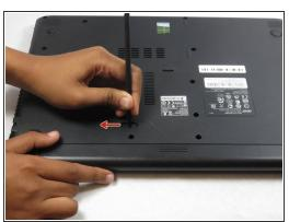
Use your finger or a spuger to pull the battery release switch.
