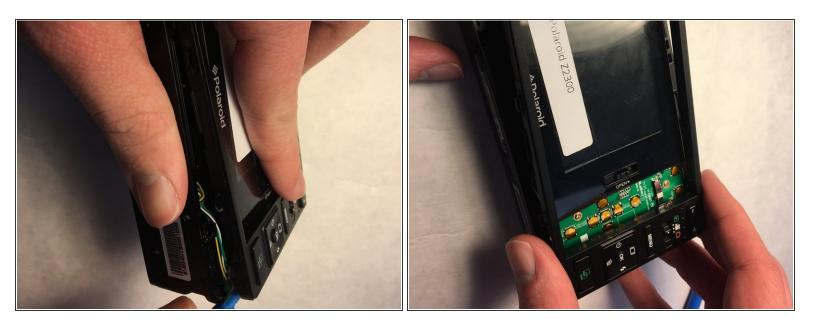
• Use a plastic opening tool to pop the control panel off, it should be easy to lift up and remove.
