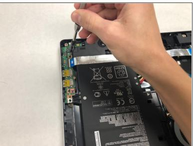
Remove the two 4.7 mm screws with the Phillips #0 screwdriver.
