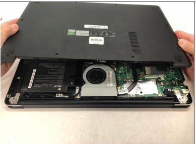
• Using a heavy-duty spudger, pry the back cover up from the frame and completely remove.
