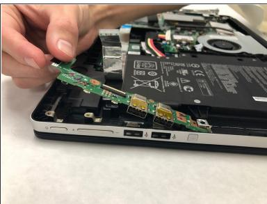
• Remove the board itself by carefully pulling the board up then away from the rest of the computer.
