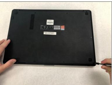
Remove the ten 10.7 mm screws using a Phillips #0 screwdriver from the back of the laptop.
