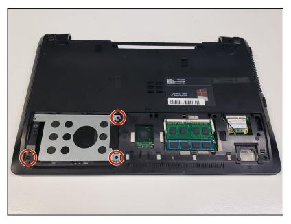
• Use a Phillips #0 screwdriver to remove the 1.5 mm screws that hold down the hard drive.
