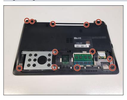
Using the the Philips #0 Screwdriver remove highlighted screws.
