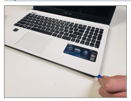
Lift keyboard panel with plastic pry tool to remove.
