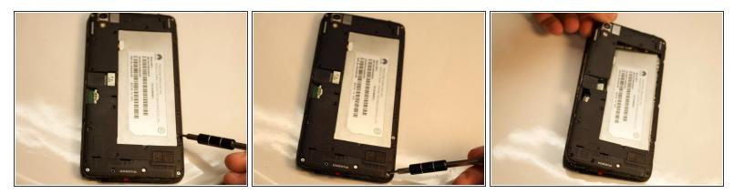
• Remove the 15 screws on the back of the device using a Phillips #000 screwdriver.
