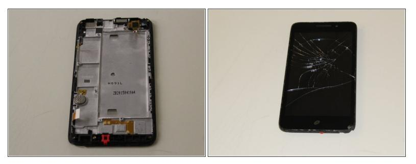
• Once the battery is removed the screen will be visible.
