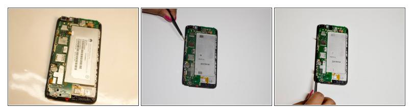
• Detach the yellow latches along the sides to remove the motherboard.
