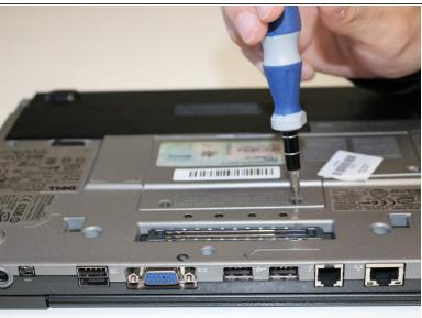
Use a Phillips #00 screwdriver to remove the three screws that secure the small "L" shaped backplate.
