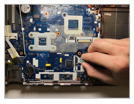
Remove the ribbon cable connecting the USB ports to the computer.
