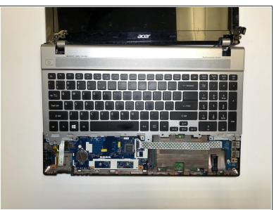
Flip the computer over and remove the touchpad cover.
