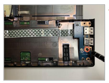
Using a Phillips #0 screwdriver, remove the one screw.
