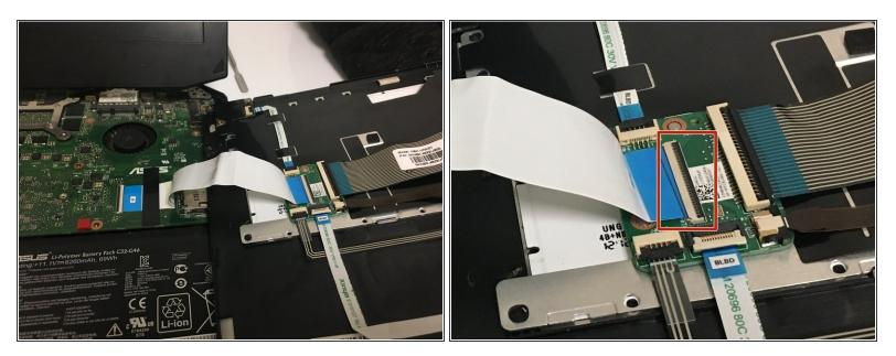
• Detach the ribbon cable by releasing the clip
