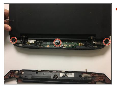
Turn the laptop over and remove the screws as shown
