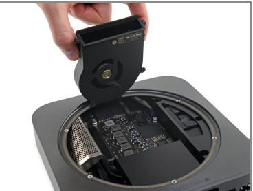
⚠ Don't try to remove the fan completely in this step—just lift it so you can access the cable underneath.
