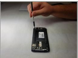
• Use a Phillips #0 screwdriver to unscrew the three 3.5mm screws in the bottom portion of the phone and put them to the side.
