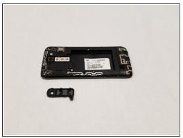
• Use a Phillips #0 screwdriver to remove the single 3.5 mm screw holding the power button and volume rocker in place and lift it out and put it to the side.
