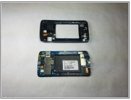
• Use a Phillips #0 screwdriver to unscrew the five 3.5 mm screws holding the housing into the device and use a spudger to pop it out of the back of the device exposing the motherboard.
