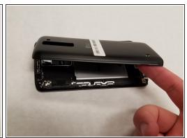
Place phone face-down and use your nail to pry the back off the back.
